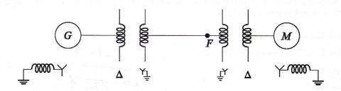
Both machines are rated 1200 kVA, 600 V with reactances of  $X_d'' = X_1 = X_2 = 10\%$  and  $X_0 = 5\%$ . Each three phase transformer is rated 1200 kVA, 600 V -  $\Delta$  / 3300 V - Y with leakage reactance of 5%. The reactance of the transmission lines are  $X_1 = X_2 = 20\%$  and  $X_0 = 40\%$  on a base of 1200 kVA and 3300 V. The reactances of the neutral grounding reactors are 5% on the base of machines. Assume the prefault current to be zero. Find
