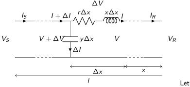
$\Delta x$  be a very small element of the line. The impedance and admittance of the section are  $z\Delta x$  and  $y\Delta x$ , respectively. From the circuit,
