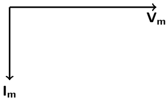
Figure: Voltage and current waveforms of Inductor
