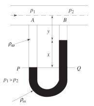
$\rho_{\rm w}$  - Density of working fluid  $\rho_{\rm m}$  - Density of manometric fluid
