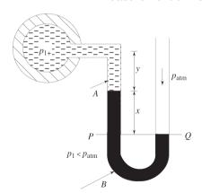
$\rho_{\rm w}$  - Density of working fluid  $\rho_{\rm m}$  - Density of manometric fluid
