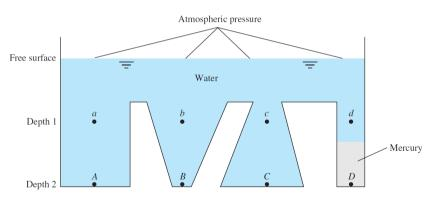
Any two points at the same elevation in a continuous mass of the same static fluid will be at the same pressure
