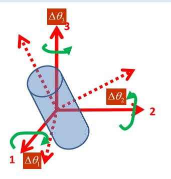
$$\frac{dL_1}{dt} = I_1 \frac{d\omega_1}{dt} + (I_3 - I_2)\omega_3\omega_2$$
