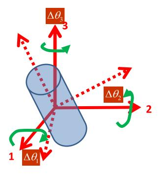
$$\tau_1 = I_1 \frac{d\omega_1}{dt} + (I_3 - I_2)\omega_3\omega_2$$
