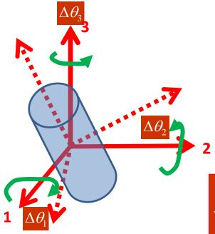
$$\Delta L_1 = I_1 \Delta \omega_1 + I_3 \omega_3 \Delta \theta_2 - I_2 \omega_2 \Delta \theta_3$$
