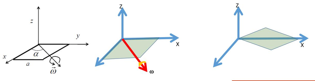
$$\begin{bmatrix} I \end{bmatrix} = \begin{pmatrix} Ma^2/3 & -Ma^2/4 & 0 \\ -Ma^2/4 & Ma^2/3 & 0 \\ 0 & 0 & 2Ma^2/3 \end{pmatrix}$$
