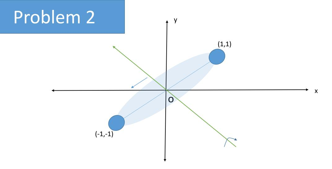
Consider no mass for the interconnecting rod between the two balls. Also consider these balls as point particles.
