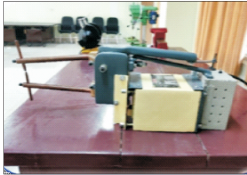
Spot Welding Machine
