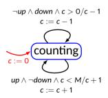
**variable**: *c* : {0, 1, ..., M} **inputs**: *up*, *down*: pure **outputs**: *count*:{0, 1, ..., M}
