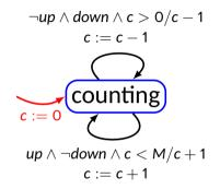
**variable**: *c* : {0, 1, ..., M} **inputs**: *up*, *down*: pure **outputs**: *count*:{0, 1, ..., M}
