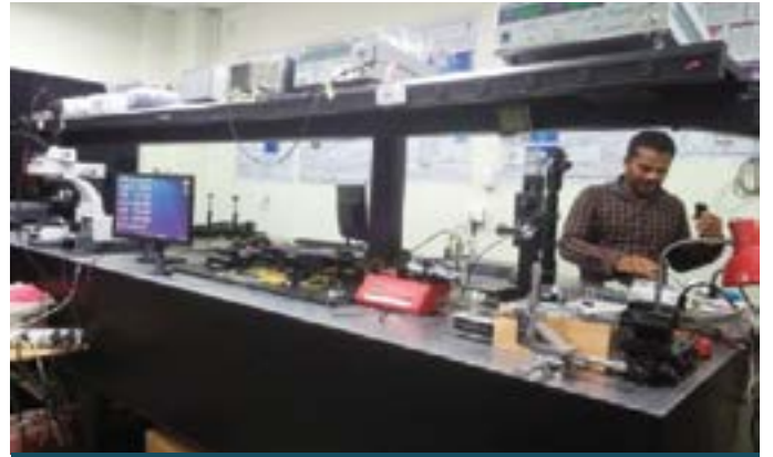
Several fiber optic devices on a vibration isolation table.
