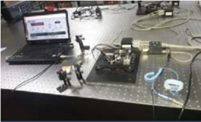
External Cavity Diode Laser automated with computer
